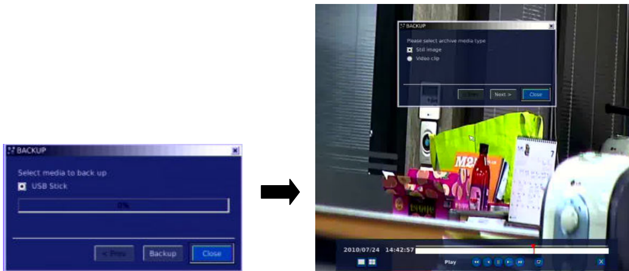
Figure 6.1.1. Still Image Archiving and Backup Screen
